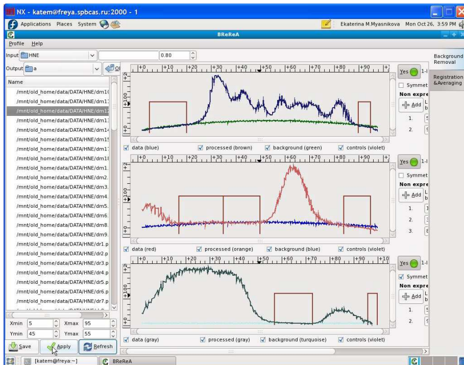
Figure 3: Background estimation. The points of support are extracted from the non-expressing areas and the initial value of background is estimated by fitting to these points. To see the initial approximating parabola on the graphs press the Refresh button. To refine the background shape press the Apply button.
