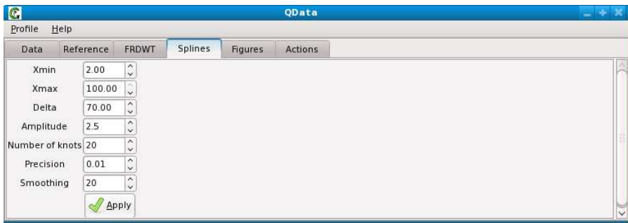
Figure 8: Screenshot of the Spline window. Input of parameters controlling the Spline feature extraction.
